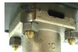
Assembly of pneumatic actuator with M5 nuts
