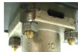
Assembly of pneumatic actuator with M5 nuts
