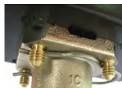
Quick assembly of pneumatic actuator with spring ring
