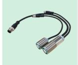
Double sheet sensor, housing diameter M18, the product is based on the ultrasonic thru-beam principle, output support 2 x DC 3-wire. The setting distance is operated by setting line, IP65, LED indicator, applied to inspections single sheet and double sheet.
