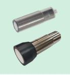
Metal housing M30 product, the max rated operating distance is 4 m, output support DC, 3-wire and analog voltage. The setting distance is operated by settingline, IP65, LED indicator, support for medium and long-range detection.
