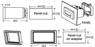
The included mounting adapter allows the counter to be fitted into existing 1" x 2" cutouts.
