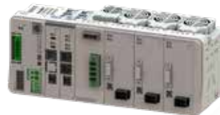
RSEL for CRS (Cartesian axis AC servo motor type)
