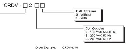
1/4" NPT, 12.5mm, 230 psi, Brass (3505) 120 VAC 50/60 Hz, without Ball / Strainer
