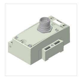
I/O module version Version Ambient temperature min./max. -10 ... 50 °C Power consumption electronics 0.05 A Max. current per channel 0.3 A Power supply for actuators 24 V DC 4 A Total current for actuators Protection class IP65 Total current of sensors max. 1,2 A Diagnosis Short circuit Weight 0.274 kg
