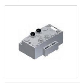
Ambient temperature min./max. -10 ... 50 °C Operational voltage electronics 24 V DC Electronics voltage tolerance -10% / +10% 24 V DC Power supply for actuators Total current for actuators 4 A Protection class IP65 Diagnosis Short circuit I/O connection M12x1, 4-pin Weight See table below
