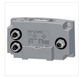
Ambient temperature min./max. -10 ... 50 °C 24 V DC Operational voltage electronics Electronics voltage tolerance -10% / +10% Power consumption electronics 0.9 A 24 V DC Operating voltage, actuators Total current for actuators 4 A IP65 Protection class Number of solenoid coils max. 128 Number of valve positions max. 110
