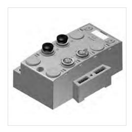
Version I/O module version Ambient temperature min./max. -10 ... 50 °C Operational voltage electronics 24 V DC Electronics voltage tolerance -10% / +10% 0.07 A Power consumption electronics Power supply for actuators 24 V DC 4 A Total current for actuators Protection class IP65
