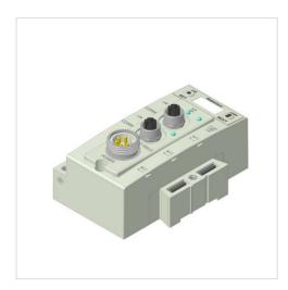
Bus coupler Version Ambient temperature min./max. -10 ... 50 °C Operational voltage electronics 24 V DC Electronics voltage tolerance -10% / +10% Power consumption electronics 0.11 A 24 V DC Operating voltage, actuators Total current for actuators 4 A Protection class IP65 Diagnosis Undervoltage I/O module extension max. 16
