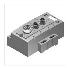
Version Bus coupler Ambient temperature min./max. -10 ... 50 °C Operational voltage electronics 24 V DC -10% / +10% Electronics voltage tolerance Power consumption electronics 0.104 A 24 V DC Operating voltage, actuators Total current for actuators 4 A Protection class IP65 Number of solenoid coils max. 128 Number of valve positions max. 110 Undervoltage Diagnosis
