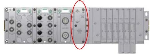
The MCM is an optional module that is installed between the node and the valve adapter module and allows the user to manually set the last octet of the IP address without the need for software configuration or the use of the integrated graphic display in the node. **If software configuration or configuration via the integrated graphic display in the node is preferred, this module is not necessary.**
