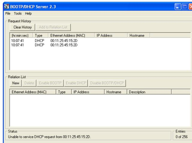
The DHCP/BOOTP setting can be enabled or disabled via the nodes integrated web server or graphical display.
